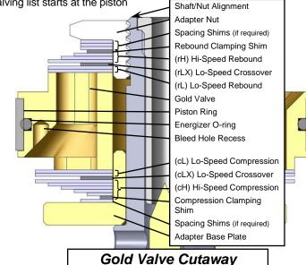
With Adapter Base Plate and Nut figure 2
